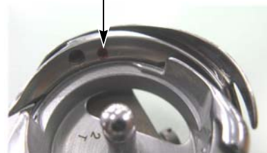
Lubrication hole (red mark)
